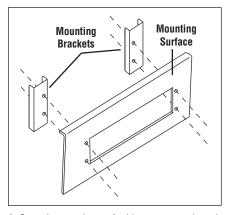
Open the two pieces of rubber cover on the unit to display the four screw holes then using four screws (M4X30) to mount the unit to the dashboard.
